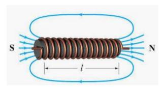
Like all magnets, the magnetic field of an activated solenoid has positive and negative poles that will attract or repel material sensitive to magnets. In a solenoid, the electromagnetic field causes the piston to either. Move backward or forward, which is how motion is created by a solenoid coil.
